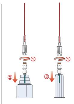
3) For further blood collections using the S-Monovette® detach the BloodCulture-Adapter from the guide sleeve of the Safety-Multifly®-Needle.
