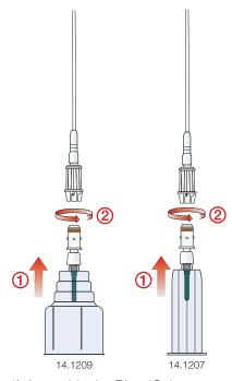
Assemble the BloodCulture-Adapter with the guide sleeve of the Safety-Multifly®-Needle already in situ.
