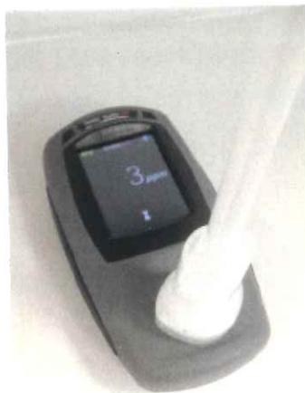
Picture of Gastrolyser used to measure hydrogen (H<sub>2</sub>) levels in breath
